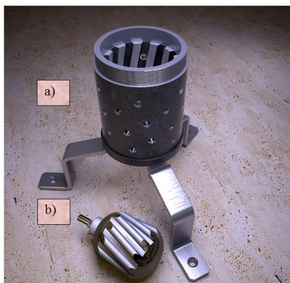
Fig. 6 . Viscometric device sensor elements; a) stator, b) rotor.
